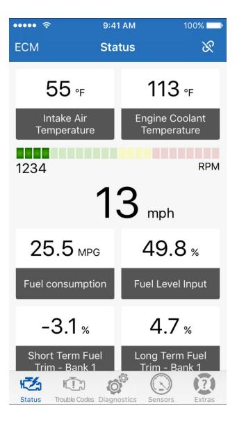
On the top left corner of the view is the Engine Control Unit (ECU) selection button. Tap the button (in the image labeled ECM) to open the ECU selection. The list contains all OBD2 compliant control units from your car.
